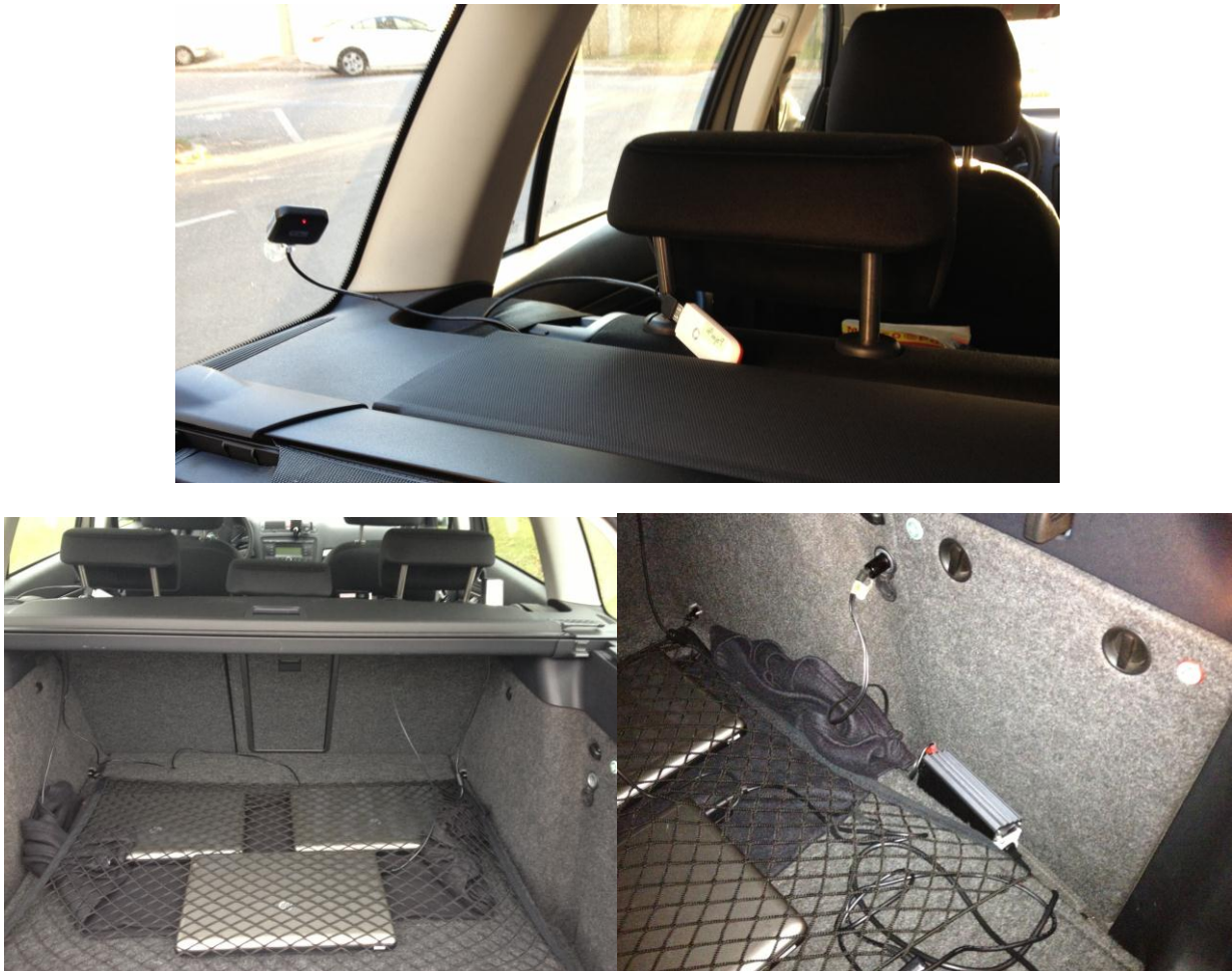
Figure 4-8: Upgraded mobile QoE measurement system deployed in a civil vehicle, showing the GPS probe (above), three QoE probes for parallel measurements of three competitive HSPA mobile networks (below left), and DC/AC power supply transformation for the QoE probes (below right) .
